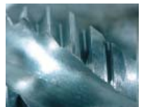
■ Cutting edge after 1.000 holes Tapping
